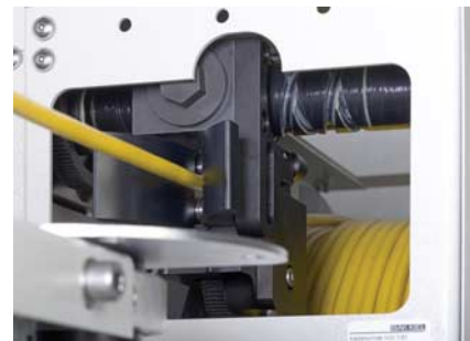
IBAK KW 180 with automatic level winding device and powerful motor
