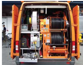
TV inspection and jetter combination
