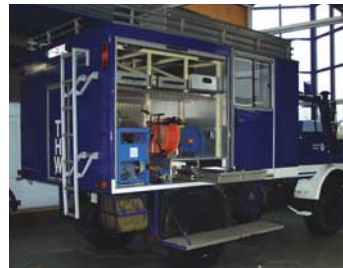
Special TV inspection outfitting
