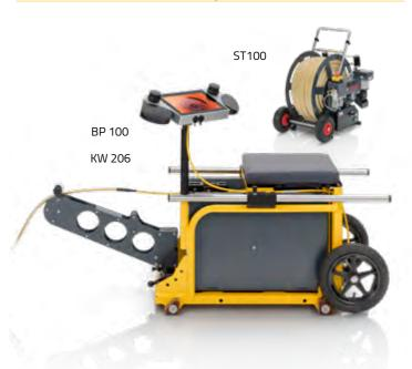
For mobile applications, the control panel BP 100 is used in combination with the KW 206/306. This device configuration ensures user-friendly operation while offering a particularly high degree of flexibility in terms of the many different possible cutting applica-
